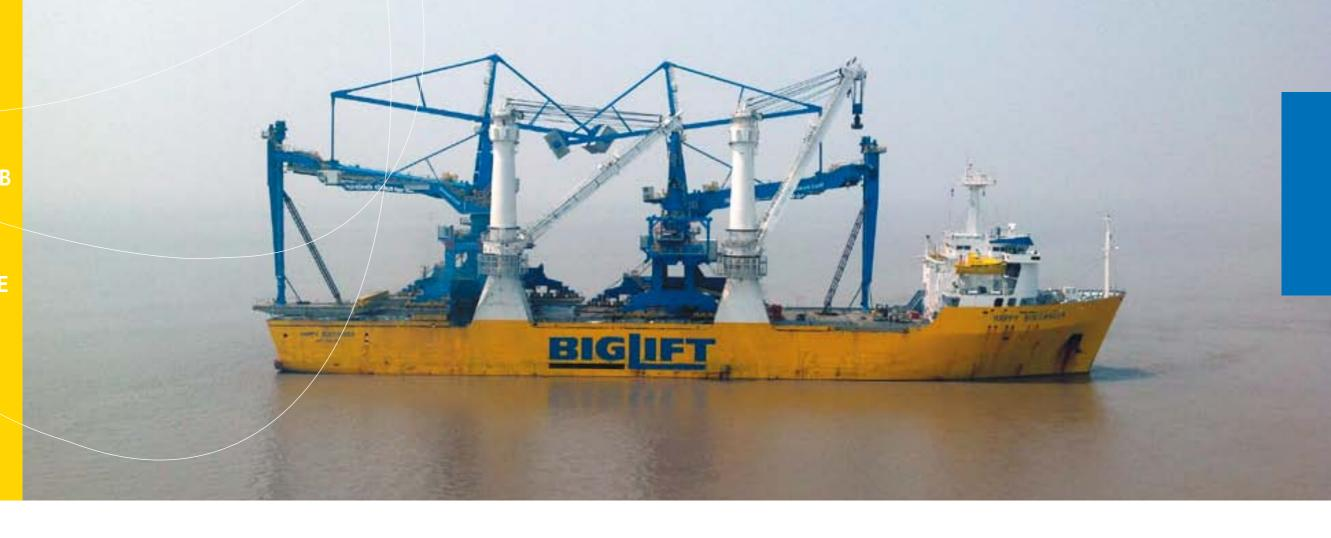
BigLift's Happy Buccaneer was contracted by Cargotec – Siwertell to transport two coal ship unloaders from Qidong, China to Jorf Lasfar, Morocco; a long voyage of almost 13,000 nm, around the Cape of Good Hope.
