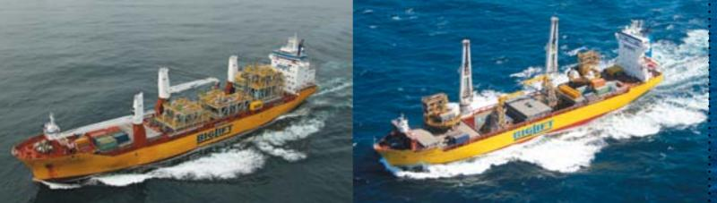
length o.a. 156.93 m registration Netherlands length p.p. 147,75 m 2 cranes each 400 mt 1 crane 120 mt breadth mld 25.60 m 17.518 mt class LLOYD'S ₹100A1 LA deadweight Finnish Ice class 1A under deck 20,892 cbm on deck 2,736 sqm Open sailing
