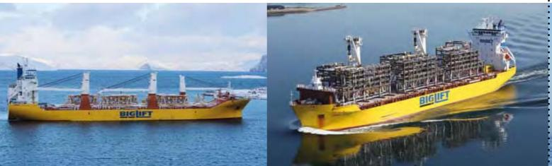
length o.a. 156.93 m registration Netherlands length p.p. 147,75 m 2 cranes each 400 mt 1 crane 120 mt breadth mld 25.60 m 17.518 mt class LLOYD'S № 100A1 LA deadweight Finnish Ice class 1A under deck 20,892 cbm on deck 2,736 sqm Open sailing
